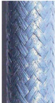
Filament winding (Fiber volume fraction: high)
