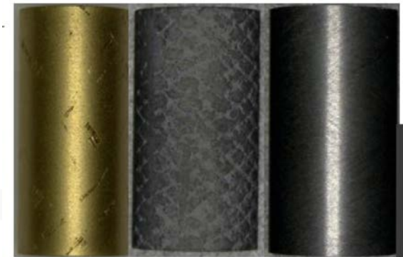
TiN on SiC/SiC SiC/SiC SiC on SiC/SiC
