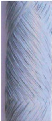
Filament winding (Fiber volume fraction: high)
